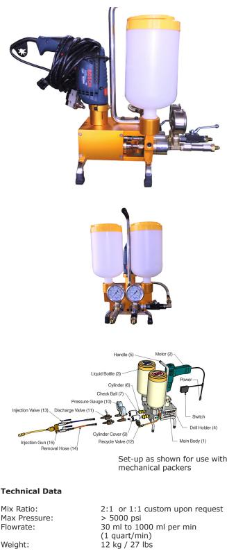
Electric Drill, adaptors/fittings and packers sold separately. Please ask your SealBoss® technician for suitable injection grouts. Viscosity range 10-1000 cps.
